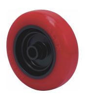
Red polyurethane tyre on black polypropylene centre.  $95^{\circ}$  shore A Temperature range:  $-25^{\circ} \div +80^{\circ}$
