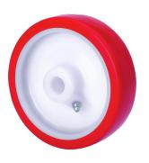
Red polyurethane tyre on white polyamide centre.95° shore A Temperature range:  $-25^{\circ} \div +80^{\circ}$
