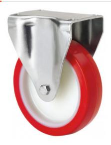
Castors with white nylon centre and red polyurethane tyre with a hardness of 90-95° Shore A. Especially indicated to support high-loads up to 600 Kg.
