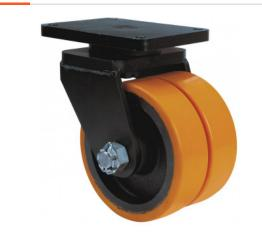
Double castors with steel centre and cast polyurethane tyre with a hardness of 95° Shore A, especially indicated to support high-loads up to 4.000 Kg.
