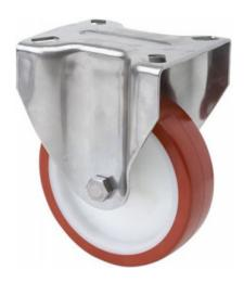
Injected polyurethane castors with stainless steel (AISI 304) components. Especially indicated to support high-loads up to 300 Kg.
