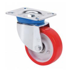
Castors with white nylon centre and red polyurethane tyre with a hardness of 90°-95° Shore A. Especially indicated to support high-loads up to 600 Kg.
