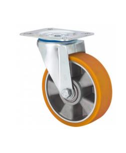
Castors wiht aluminium centre and cast polyurethane tyre with a hardness of 95° Shore A. Especially indicated to support high-loads up to 400 Kg.
