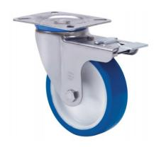
Castors with white polypropylene centre and soft blue injected polyurethane tyre with a hardness of 80° Shore A. Especially indicated to support high-loads up to 250 Kg.
