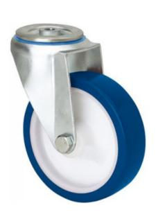
Castors with white polypropylene centre and soft blue injected polyurethane tyre with a hardness of 80° Shore A. Especially indicated to support high-loads up to 250 Kg.
